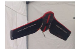
SenseFly EbeeX MTOW: 1,6kg SODA 3D RGB NIR camera Thermomap (Termica) Modelli 2D/3D
